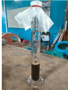
Gambar 1 Pengujian kadar lumpur
