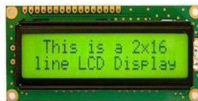
**Gambar 3. LCD (Liquid Crystal Display)**
